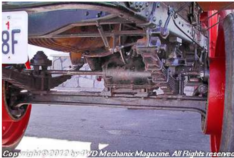
Nash-Quad trucks were available in two- and four-wheel steer. This chassis is front steering only. Differentials with "automatic lockers" and front-rear drive shafts make up the 4WD system.
