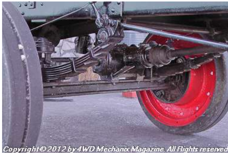
Portal axles? This 1918 truck has its differential and driveshafts above the iron beam axle. The iron beam is below the semi-elliptic leaf springs. Ground clearance is ample. Driveshafts are well out of the way.
